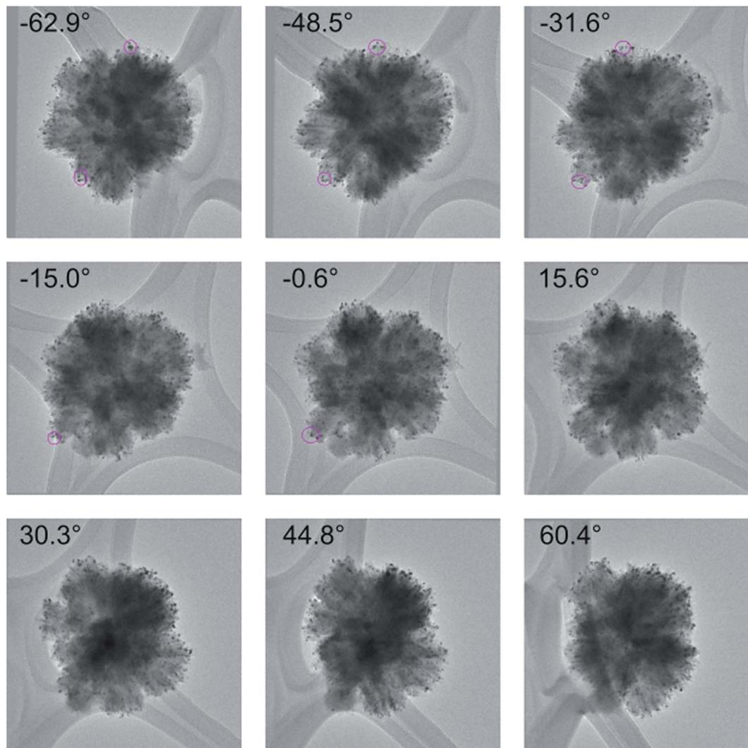
Fig. 2 A selection of images used for the TEM tilt series of the 5% Au-RANR catalyst after *in situ* PXRD measurements. Selected Au nanoparticles were tracked using fiducial tracking during the rotation to confirm their positions. The reconstruction video can be accessed in the ESI.†
