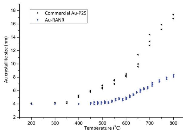
Fig. 3 Au crystallite sizes of the commercial Au-TiO<sub>2</sub> and Au-RANR catalysts determined from Rietveld refinement from *in situ* PXRD.
