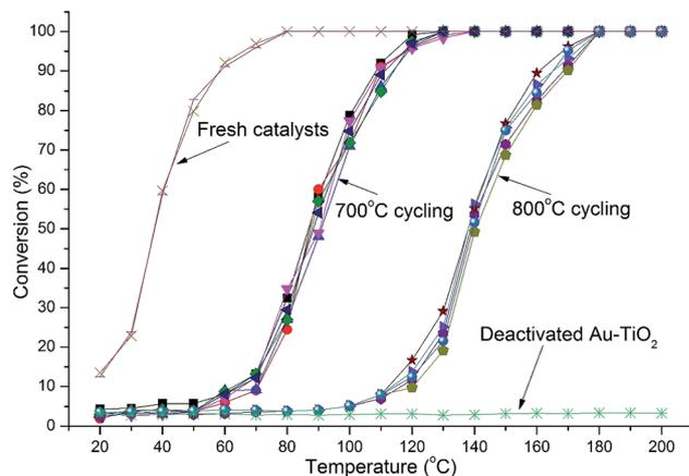
Fig. 4 Light-off curves for catalysts with 1.2% Au-RANR and commercial Au-TiO<sub>2</sub> after multiple 700 and 800 °C heating cycles (10 cycles in total).
