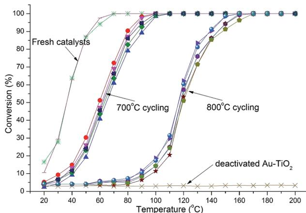
Fig. 5 Light-off curves for catalysts with 5% Au-RANR and commercial Au-TiO<sub>2</sub> catalyst after multiple 700 and 800 °C heating cycles (10 cycles in total).
