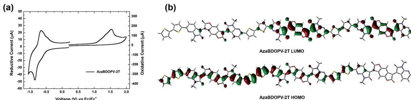
Fig. 3 (a) Cyclic voltammogram of the polymer AzaBDOPV-2T in thin film prepared by drop-casting the polymer solution ( $1 \text{ mg mL}^{-1}$  in CHCl<sub>3</sub>) on a glassy carbon electrode; (b) calculated molecular orbitals of the AzaBDOPV-2T trimer at the b3lyp/6-31g(d) level.
