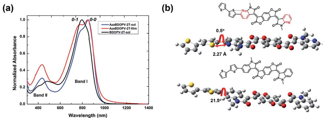
Fig. 2 (a) The absorption spectra of the polymer BDOPV-2T in dilute solution ( $10^{-5}$  M), AzaBDOPV-2T both in dilute solution ( $10^{-5}$  M) and in thin film; (b) DFT-optimized geometries of AzaBDOPV-2T and BDOPV-2T fragments. Alkyl chains were replaced by methyl groups for simplicity (geometries were optimized at the b3lyp/6-311g(d,p) level).
