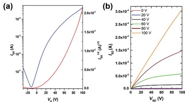
Fig. 4 (a) Transfer and (b) output characteristics of an AzaBDOPV-2T device tested under ambient conditions ( $L = 5 \mu\text{m}$ ,  $W = 100 \mu\text{m}$ ,  $C_i = 3.5 \text{ nF cm}^{-2}$ ), measured  $V_T = 40 \text{ V}$ .
