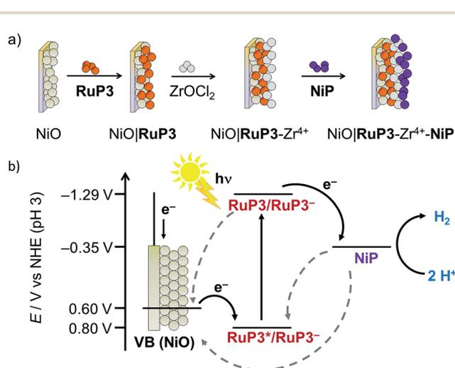
Fig. 2 (a) Supramolecular dye-catalyst assembly on photocathode: layer-by-layer deposition of **RuP3**, Zr<sup>4+</sup> and **NiP** on p-type NiO photocathode (see text for details). (b) Energy diagram of the NiO photocathode assembly showing the proposed electron transfer mechanisms (reductive quenching) as black solid arrows and possible recombination pathways as grey dashed arrows between p-NiO, **RuP3** and **NiP**.
