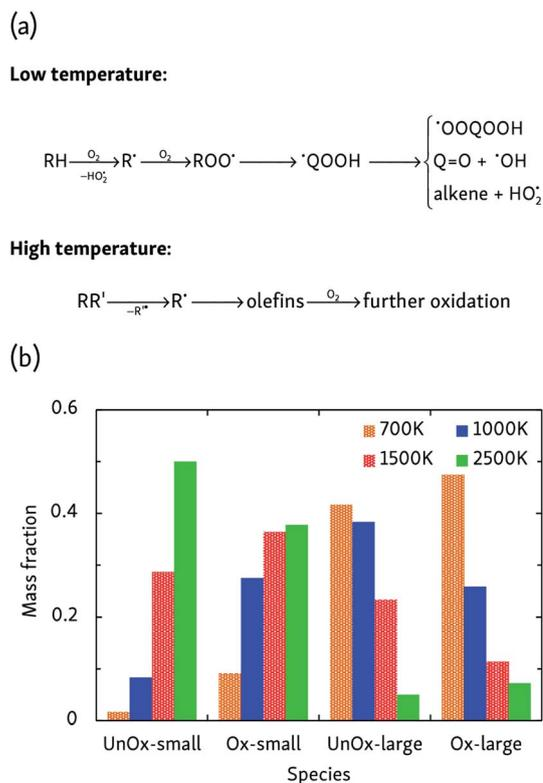
Fig. 3 (a) Limiting temperature-dependent initial oxidation mechanisms, and (b) products of the constant-density CVHD *n*-dodecane oxidation simulations at different temperatures. Unox species do not contain oxygen, whereas Ox do; large products are C<sub>3</sub> or heavier. The mass fraction is that of carbon only, and reflects how carbon is distributed over the various species.
