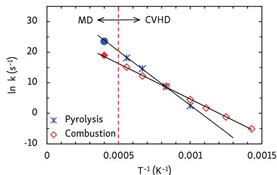
Fig. 5 Arrhenius plots of the apparent first order rate constants of *n*-dodecane pyrolysis and combustion as obtained from CVHD simulations. Filled symbols at 2500 K are unbiased MD simulations that were not included in the fit.
