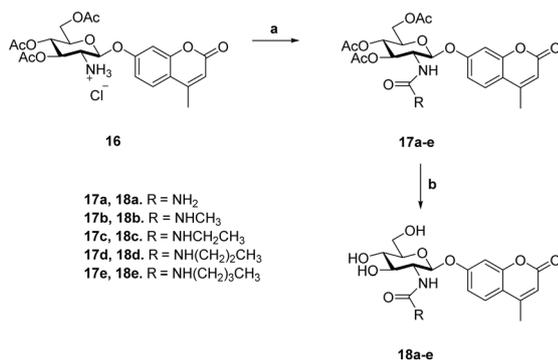
**Scheme 2** Synthesis of 4-methylumbelliferyl fluorogenic substrates **18a–e**. (a) R-NCO, NEt<sub>3</sub>, CH<sub>3</sub>CN; (b) (i) NaOMe, MeOH; (ii) Dowex 50-H<sup>+</sup>.
