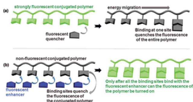
Fig. 1 Using conjugated polymers as fluorescent sensors.
