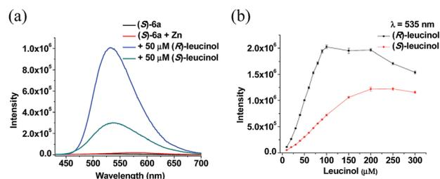
Fig. 2 Fluorescent spectra of (S)-6 ( $5.0 \times 10^{-5}$  M) + Zn(II) ( $1.0 \times 10^{-4}$  M) in CH<sub>2</sub>Cl<sub>2</sub> with 1 equiv. of (R)- and (S)-leucinol (a). Fluorescent intensities at  $\lambda = 535$  nm versus leucinol concentrations (error bars are from three independent measurements) (b). ( $\lambda_{ex} = 355$  nm, slit: 3/3 nm).
