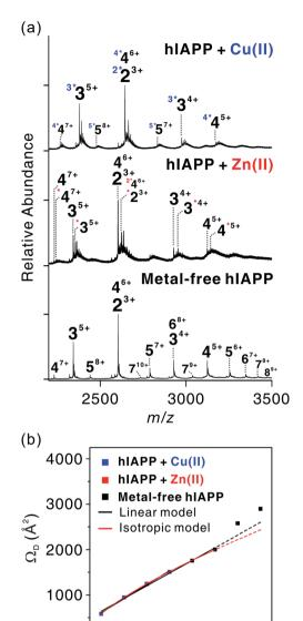
Fig. 4 Assembly mechanism of hIAPP oligomers. (a) ESI-MS for oligomeric hIAPP incubated with and without metal ions. z-Charged nmer ion is denoted as  $n^{z+}$ , and left superscript with asterisks k ( $^k*$ ) indicates k metal ions included in the oligomers. (b) Correlations between oligomeric state (n) and  $\Omega_D$  of  $n^{n+1}$  ions for experimentally detected oligomers. Calibration curve of the oligomers is available in Fig. S13.†
