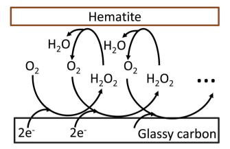
Fig. 4 Graphical representation of the oxygen reduction/regeneration cycle at the hematite modified glassy carbon electrode.
