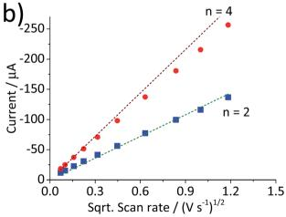
Fig. 2 (a) Cyclic voltammograms of a glassy carbon electrode modified with  $2.4 \times 10^{-5}$  g cm $^{-2}$  of hematite nanoparticles in  $O_2$  saturated 20 mM KCl at the scan rate varied from 1.4 V s $^{-1}$  to 0.005 V s $^{-1}$ . (b) Plots of peak current as a function of the square root of the scan rate for the hematite modified electrode (a) and for the bare electrode (b) Dashed lines are calculated using eqn (5) for the 2-electron and the 4-electron reactions.
