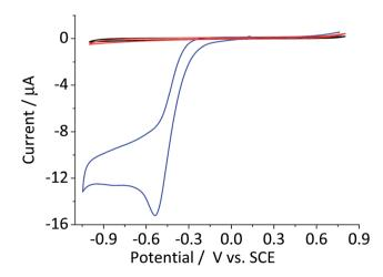
Fig. 3 Cyclic voltammetric curves of a bare glassy carbon electrode (red) and that modified with  $2.4 \times 10^{-5}$  g cm $^{-2}$  of hematite nanoparticles in N<sub>2</sub> saturated 20 mM KCl with 1.5 mM H<sub>2</sub>O<sub>2</sub> collected at the scan rate of  $0.01\,\text{V}$  s $^{-1}$ . Black line illustrates a cyclic voltammetric curve of bare glassy carbon in the same KCl solution without H<sub>2</sub>O<sub>2</sub>.
