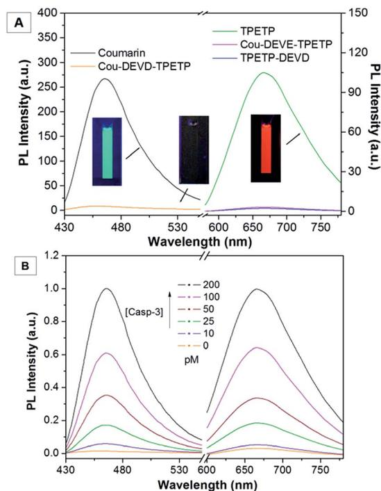
Fig. 1 (A) Photoluminescence (PL) spectra of Cou, TPETP-N<sub>3</sub> and Cou-DEVD-TPETP (10  $\mu\text{M}$ ) in DMSO/PBS buffer (v/v = 1/99). (B) PL spectra of Cou-DEVD-TPETP (10  $\mu\text{M}$ ) upon incubation with different concentrations of caspase-3 ( $\lambda_{\text{ex}}$ : 405 nm, emission collected from 430–550 nm is from Cou-DEVD and that at 600–780 nm is from the TPETP residue).
