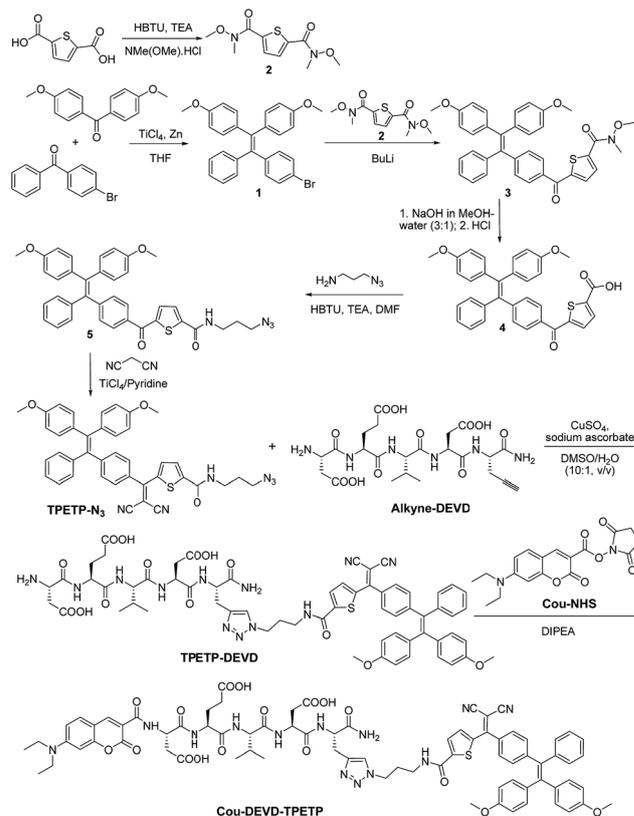
**Scheme 2** Synthetic route to the probe Cou-DEVD-TPETP. HBTU: *O*-(benzotriazol-1-yl)-*N,N,N',N'*-tetramethyluronium hexafluorophosphate; TEA: triethylamine; TiCl<sub>4</sub>: titanium(iv) chloride; Zn: zinc; THF: tetrahydrofuran; BuLi: butyllithium; DMF: *N,N*-dimethylformamide; DIPEA: *N,N*-diisopropylethylamine; Cou-NHS: 7-(diethylamino)coumarin-3-carboxylic acid *N*-succinimidyl ester.
