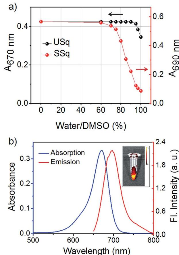
Fig. 1 (a) Changes in the absorption spectra of USq and SSq ( $2 \mu\text{M}$ ) in DMSO upon increasing the content of water from 0–100%. (b) UV/Vis absorption (blue curve) and emission spectra (red curve,  $\lambda_{\text{ex}} = 640 \text{ nm}$ ) of USq ( $2 \mu\text{M}$ ) in 96% phosphate buffer (pH 7.8)/DMSO mixture. Inset shows false-color pixel intensity map image of USq ( $\lambda_{\text{ex}} = 640 \text{ nm}$ ) in 96% phosphate buffer/DMSO mixture.
