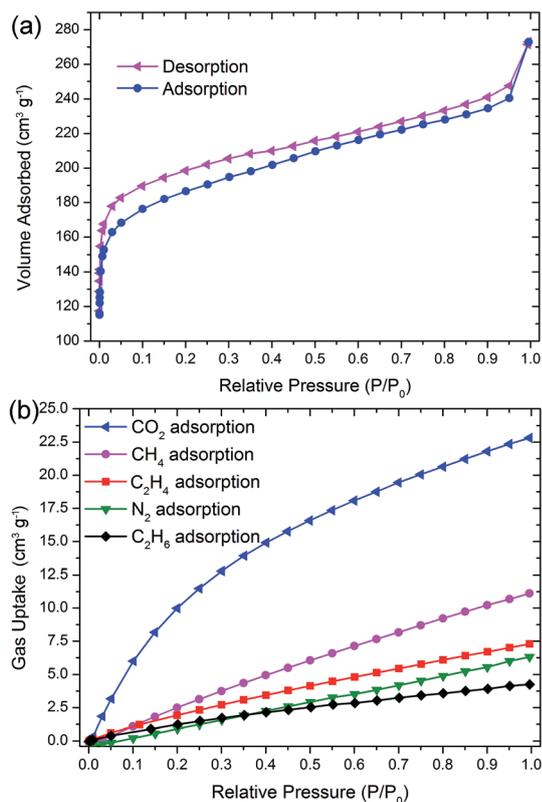
Fig. 5 Gas sorption isotherms of ozone-treated PKU-15. (a)  $\text{N}_2$  sorption isotherms at 77 K. (b)  $\text{CO}_2$ ,  $\text{CH}_4$ ,  $\text{C}_2\text{H}_4$ ,  $\text{N}_2$  and  $\text{C}_2\text{H}_6$  adsorption isotherms at 273 K.  $P_0$  represents the standard pressure.
