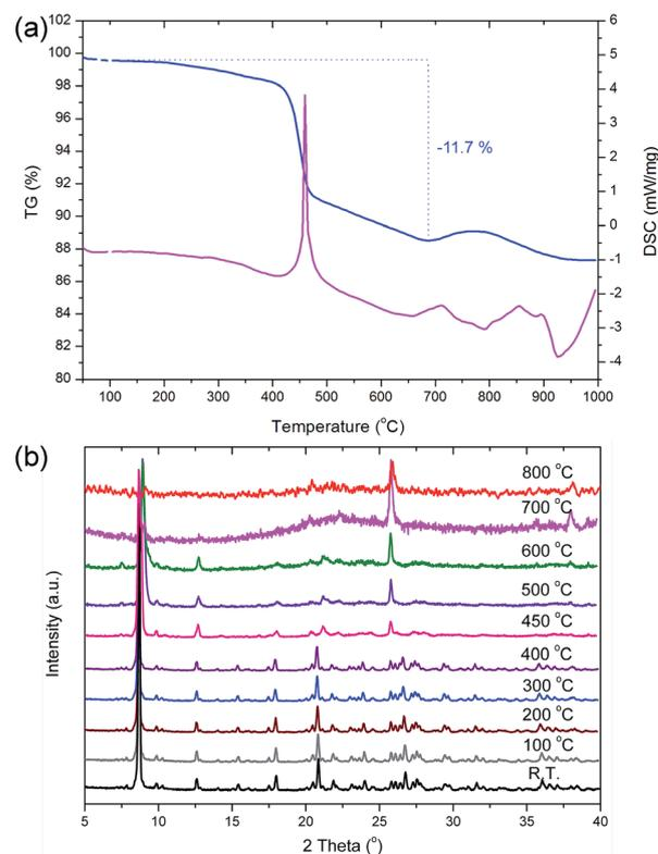
**Fig. 4** The thermal properties of as-synthesised PKU-15. (a) TG-DSC curves of as-synthesised PKU-15. The TG curve is drawn in blue, and the DSC curve is in purple. (b) *In situ* variable-temperature powder X-ray diffraction patterns of as-synthesised PKU-15 heated from room temperature (R.T.) to 800 °C.
