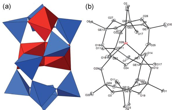
Fig. 1  $(\text{Ge,Si})_{12}\text{O}_{31}$  cluster in PKU-15. (a) Polyhedral and (b) thermal ellipsoidal (50%) representations of the cluster. In (a), the  $\text{GeO}_5$  trigonal bipyramids are drawn in red, and the  $\text{GeO}_4$  tetrahedra are in blue. In (b), the tri-coordinated oxygen atom in the cluster is drawn in red.
