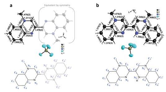
Fig. 2 Crystallographic structures of  $\mathbf{1}^{2+}/\mathbf{1}^0$ -H<sup>+</sup>: view of the asymmetric unit of [MBqn<sup>2+</sup>](BF<sub>4</sub>)<sub>2</sub>, [ $\mathbf{1}^{2+}$ ](BF<sub>4</sub>)<sub>2</sub> (a) and [MBqn<sup>0</sup>-H<sup>+</sup>]BF<sub>4</sub>, [ $\mathbf{1}^0$ -H<sup>+</sup>]BF<sub>4</sub> (b). Salient C-N and C-C bond lengths are indicated.
