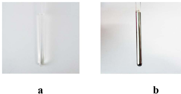
Fig. 6 Photos of 2^{2+} \cdot 2PF_6^- (4.5 mM L -1 ) taken 10 min (a) and 10 h (b) after treatment with 4 molar equiv. of AgNO 3 in a mixture of CD 3 CN, D 2 O, and ND 3 ·D 2 O (25–28% by mass) (1/0.4/0.007, v/v/v) at 323 K.
