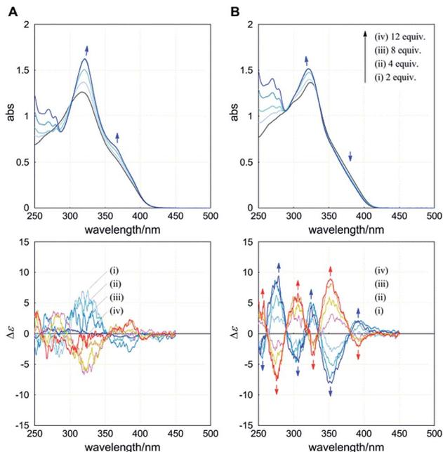
Fig. 6 UV (upper) and CD (lower) spectra of **1** (**A**) ( $7.5 \times 10^{-5}$  M) and **2** (**B**) ( $9.9 \times 10^{-5}$  M) in the presence of ( $R$ )<sub>2</sub>-**6** (blue lines) or ( $S$ )<sub>2</sub>-**6** (red lines) [0 (black, host only), 2, 4, 8 and 12 equiv.]. All spectra were measured in dichloromethane at 293 K.
