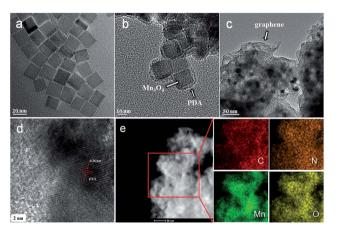
Fig. 1 TEM images of (a) the  $\rm Mn_3O_4$  nanocrystals, (b) the  $\rm Mn_3O_4$ @PDA nanocrystals, and (c and d) the GMNCs at different magnifications. (e) Dark-field TEM image and the corresponding EDS elemental mapping images of the GMNCs for carbon (C), nitrogen (N), manganese (Mn) and oxygen (O).
