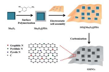
Scheme 1 Schematic illustration on the preparation of the GNS@MnO@N-doped carbon composites (GMNCs).
