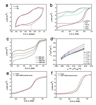
Fig. 5 (a) CV curves of the GMNCs in Ar-saturated and  $O_2$ -saturated 0.1 M KOH. (b) ORR polarization curves for the GMNCs, Pt/C, Mn $_3$ O $_4$ , MnO and GNCs at 1600 rpm. (c) ORR polarization curves of the GMNCs at different rotating speeds. (d) K–L plots of the GMNCs at different potentials. ORR polarization curves of the GMNCs (e) and Pt/C (f) before and after 10 000 potential cycles.
