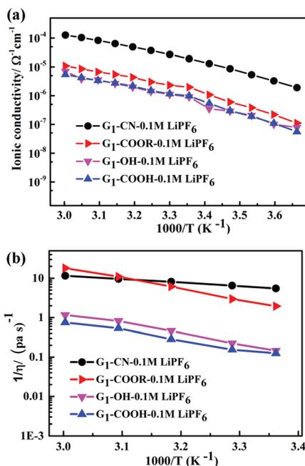
Fig. 2 (a) Temperature dependent ionic conductivity and (b) fluidity ( $\eta^{-1}$ ) of G<sub>1</sub> dendrimers with different peripheral functional groups.
