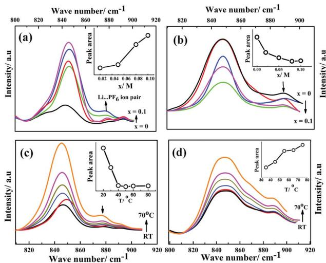
Fig. 3 FTIR spectra of G<sub>1</sub>-CN-LiPF<sub>6</sub> (a) and G<sub>1</sub>-COOR-LiPF<sub>6</sub> (b) at different salt concentrations [x = 0 (black), 0.01 (red), 0.02 (magenta), 0.05 (green), 0.1 (blue)]. FTIR spectra of G<sub>1</sub>-CN-LiPF<sub>6</sub> (c) and G<sub>1</sub>-COOR-LiPF<sub>6</sub> (d) at different temperatures (T = RT to 70 °C, with x = 0.1) [T = RT (black), 30 °C (red), 40 °C (blue), 50 °C (green), 60 °C (magenta), 70 °C (orange)].
