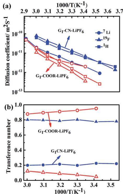
Fig. 4 (a) Self-diffusion coefficients of <sup>1</sup>H (squares), <sup>19</sup>F (triangles), <sup>7</sup>Li (circles) at various temperatures for G<sub>1</sub>-CN-0.1 M LiPF<sub>6</sub> (blue, with closed symbols) and G<sub>1</sub>-COOR-0.1 M LiPF<sub>6</sub> (red, with open symbols). (b) <sup>7</sup>Li and <sup>19</sup>F transference numbers of G<sub>1</sub>-CN-0.1 M LiPF<sub>6</sub> (blue) and G<sub>1</sub>-COOR-0.1 M LiPF<sub>6</sub> (red) at various temperatures.
