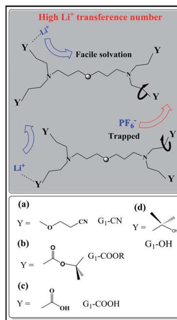
Fig. 1 Schematic representation of ion transport mechanism in  $G_1$ -PETIM dendrimers with different peripheral functional groups: (a)  $G_1\text{-CN}$ , (b)  $G_1\text{-COOR}$ , (c)  $G_1\text{-COOH}$ , (d)  $G_1\text{-OH}$ .
