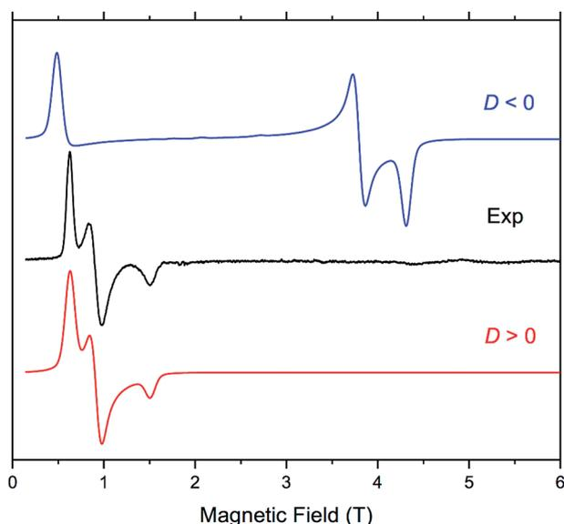
Fig. 4 EPR spectrum of **TAN@1** at 53.2 GHz and 4.5 K (black trace) accompanied by powder-pattern simulations (colored traces) using the following spin Hamiltonian parameters:  $S = 3/2$ ;  $|E/D| = 0.125$ , and  $g = [2.57, 2.57, 2.63]$ . Blue trace:  $D < 0$ ; red trace:  $D > 0$ . The rhombicity factor represents the upper bound since it is correlated with the  $g_x$  and  $g_y$  value.
