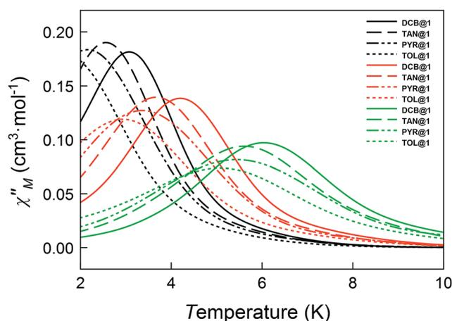
Fig. 6 Temperature dependence of  $\chi_M''$  of **DCB@1**, **TAN@1**, **TOL@1** and **PYR@1** in a dc applied static field of 1000 G and under a  $\pm 5.0$  G oscillating field at 672 (black), 2043 (orange) and 10 000 Hz (green) frequencies.
