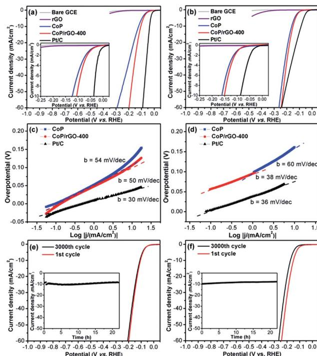
Fig. 2 Electrochemical HER activity of  $\text{CoP}/\text{rGO}-400$ . (a) LSV curves, (c) Tafel slopes and (e) durability test in  $0.5 \text{ M H}_2\text{SO}_4$  solution; (b) LSV curves, (d) Tafel slopes and (f) durability test in  $1 \text{ M KOH}$  solution. Insets in (e) and (f): time-dependent current density curves under static overpotentials of 105 mV in  $0.5 \text{ M H}_2\text{SO}_4$  and 150 mV in  $1 \text{ M KOH}$  solution, respectively.
