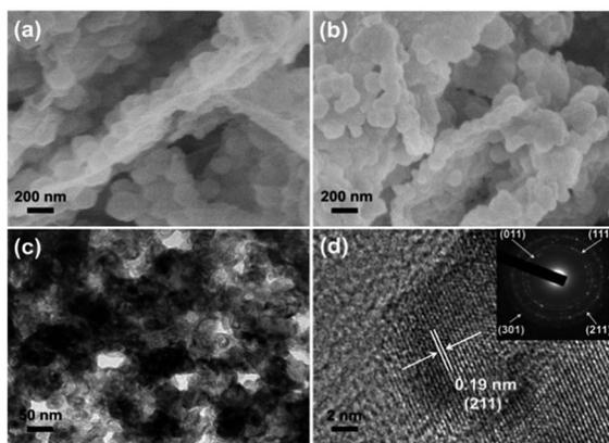
Fig. 1 Scanning electron microscope (SEM) images of (a) ZIF-67/GO and (b)  $\text{CoP}/\text{rGO}-400$ . (c) Transmission electron microscopy (TEM) and (d) high-resolution TEM images of  $\text{CoP}/\text{rGO}-400$  (inset in (d): SAED pattern for CoP nanocrystal).
