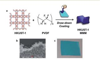
Fig. 1 Schematic depicting the fabrication of mixed-matrix membranes of HKUST-1. (a) 3-dimensional structure of HKUST-1, chemical structure of polyvinylidene difluoride, and schematic representing the MMM fabrication process, (b) SEM image of 67-HKUST-1 MMM and (c) picture of 67-HKUST-1 MMM.
