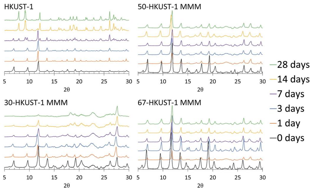
Fig. 4 PXRD patterns of 30-HKUST-1, 50-HKUST-1, and 67-HKUST-1 MMMs, compared to HKUST-1,<sup>31</sup> aged for 0, 1, 3, 7, 14, and 28 days at 90% RH at 25 °C.
