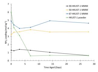
Fig. 2 Ammonia loading for HKUST-1 (powder) and HKUST-1 MMMs. Different HKUST-1 loadings after aging at 90% RH and 25 °C for various amounts of time are shown.
