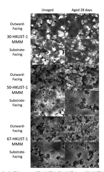
Fig. 3 SEM images of 30-HKUST-1, 50-HKUST-1, and 67-HKUST-1 shown from the outward-facing (MOF dominant) side and substrate-facing (polymer dominant) side before (left) and after (right) aging at 90% RH at 25  $^{\circ}$ C for 28 days.
