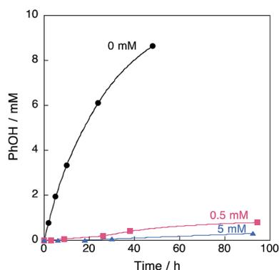
Fig. 6 Time profiles of formation of phenol in the reaction of benzene with 30 wt% aqueous  $\text{H}_2\text{O}_2$  in the presence of 1 and DMPO (0, 0.5, 5 mM) in acetone at 298 K. The concentrations are  $[\text{C}_6\text{H}_6] = 2.1 \text{ M}$ ,  $[\text{H}_2\text{O}_2] = 2.1 \text{ M}$ ,  $[\text{H}_2\text{O}] = 0.4 \text{ M}$  and  $[[\text{Cu}^{\text{II}}(\text{tmpa})]^{2+}] = 67 \mu\text{M}$  (4.75 mL).
