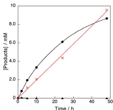
Fig. 3 Time profiles of formation of phenol (black circle) and *p*-benzoquinone (black triangle) in the hydroxylation of benzene, and formation of *p*-benzoquinone (red cross) in the oxidation of phenol with 30 wt% aqueous H<sub>2</sub>O<sub>2</sub> catalysed by 1 in acetone at 298 K; [C<sub>6</sub>H<sub>6</sub>] or [PhOH] = 2.1 M, [H<sub>2</sub>O<sub>2</sub>] = 2.1 M, [Cu<sup>II</sup>(tmpa)]<sup>2+</sup> = 67 μM in acetone (4.75 mL).
