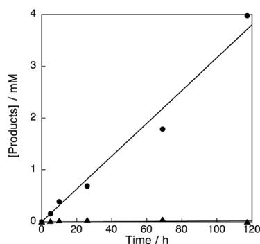
Fig. 8 Time profiles of formation of phenol (circle) and *p*-benzoquinone (triangle) in the hydroxylation of benzene (2.1 M) with 30 wt% aqueous H<sub>2</sub>O<sub>2</sub> (2.1 M) catalysed by [Cu<sup>II</sup>(tmpa)]<sup>2+</sup>@Al-MCM-41 (1.0 μM) in acetone (4.75 mL) at 298 K.
