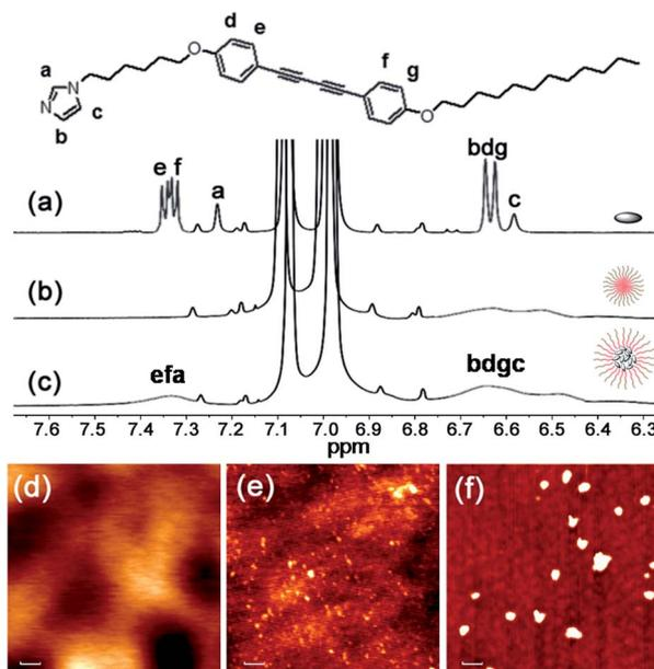
**Fig. 2** Characterizations of **P-M**: partial <sup>1</sup>H NMR spectra (400 MHz, room temperature) of (a) **M**, (b) **P** and (c) **P-M** in toluene-*d*<sub>8</sub>. The tiny peaks without labels are assigned to satellite peaks from the solvent. AFM images of (d) **M**, (e) **P** and (f) **P-M** spun from toluene solution, respectively. Scale bar: 100 nm.
