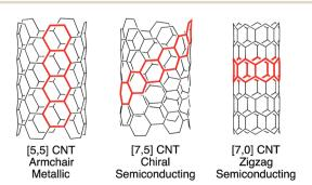
Fig. 1 Carbon nanotubes are classified as armchair, chiral, or zigzag based upon their structure. Each type has differing electronic properties.
