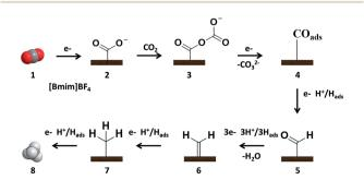
Fig. 4 CO<sub>2</sub> reduction mechanism schematic diagram at NGM/CP electrode.
