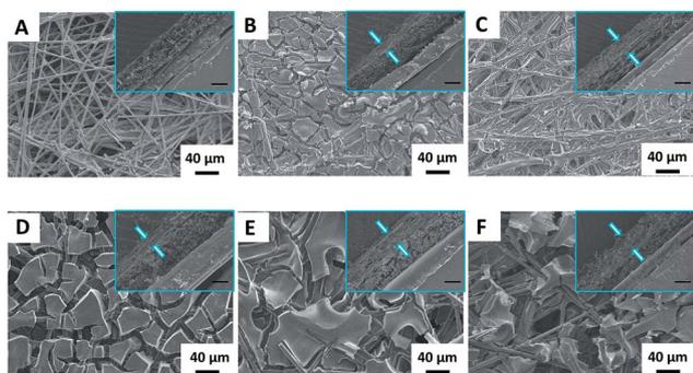
**Fig. 2** The SEM images of the NGM/CP electrodes. The inset in each image shows the thickness of the NGM on the NGM/CP electrode (scale bar, 30  $\mu\text{m}$ ). (A) CP (heated at 1000  $^\circ\text{C}$  in an argon (Ar) atmosphere for 2 h), (B) NGM-1/CP, (C) NGM-2/CP, (D) NGM-3/CP, (E) NGM-4/CP and (F) NGM-5/CP.
