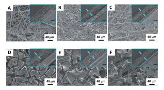
Fig. 2 The SEM images of the NGM/CP electrodes. The inset in each image shows the thickness of the NGM on the NGM/CP electrode (scale bar, 30  $\mu m$ ). (A) CP (heated at 1000 °C in an argon (Ar) atmosphere for 2 h), (B) NGM-1/CP, (C) NGM-2/CP, (D) NGM-3/CP, (E) NGM-4/CP and (F) NGM-5/CP.
