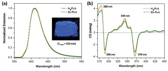
Fig. 3 (a) The fluorescence emission spectra of  $H_4PLA$  and Zn-PLA in the solid state ( $\lambda_{ex} = 350$  nm). Notice that the emission spectra of  $H_4PLA$ and Zn-PLA are identical. The inset shows the solid-state fluorescence image of the bulk sample of Zn-PLA when exposed to UV irradiation at 350 nm. (b) The solid-state CD spectra of H<sub>4</sub>PLA and Zn-PLA
