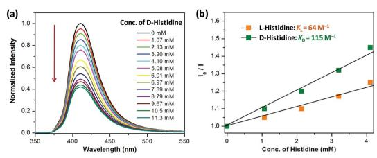
Fig. 5 (a) Quenching of the fluorescence of Zn-PLA with an increasing concentration of p-(+)-histidine in water ( $\lambda_{ex} = 350$  nm). (b) The Stern–Volmer quenching plots for p-(+)- and L-(-)-histidine.
