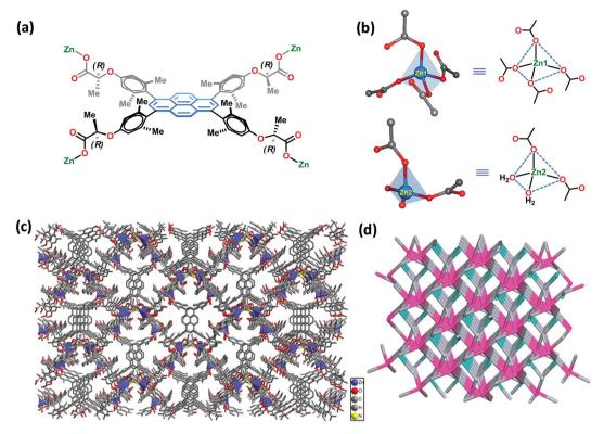
Fig. 2 (a) The coordination modes of the carboxylate groups in PLA and (b) the coordination environment of Zn1 and Zn2 in Zn-PLA. (c) The crystal packing diagram of Zn-PLA along the a-axis. (d) The simplified topology of the Zn-PLA network.
