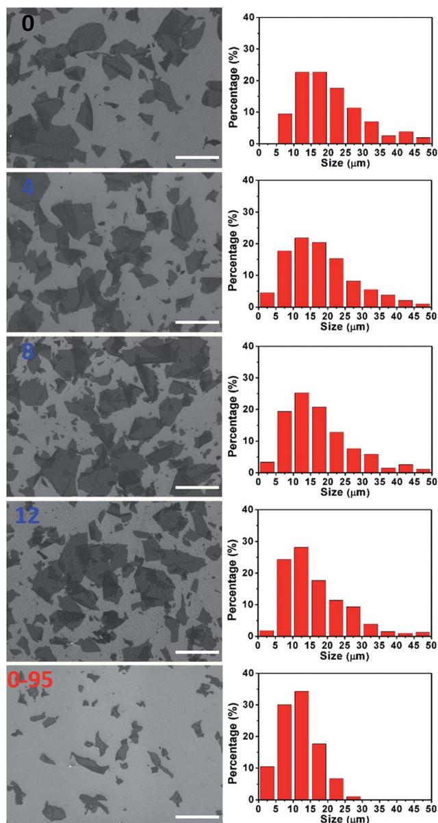
Fig. 3 Typical SEM images and corresponding histograms of GO size distributions (right to the SEM image) of GO- $n$  and GO-0-95 samples; the values of  $n$  are depicted in the panels; scale bar, 50  $\mu\text{m}$ . The histograms of GO size distributions were obtained by counting more than 200 sheets for each sample.
