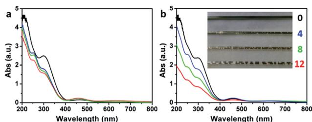
Fig. 7 UV-Vis spectra of (a) fresh H<sub>2</sub>SO<sub>4</sub> solutions of KMnO<sub>4</sub> containing 0 (black), 4 (blue), 8 (green), and 12 mL (red) water at 0 °C, respectively, and (b) after keeping them at 40 °C for 2 h. Inset in (b) shows the photographs of the corresponding solutions in capillary tubes.
