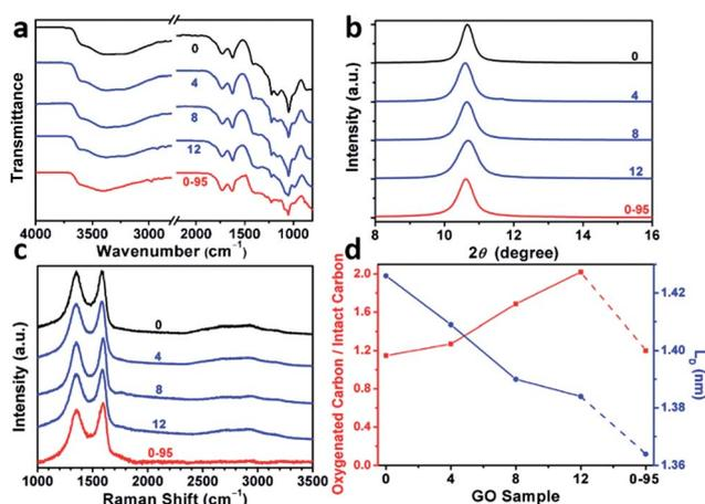
Fig. 2 (a) ATR-FTIR spectra, (b) XRD patterns, (c) 514.5 nm excited Raman spectra, (d) atomic ratio of oxygenated carbons/intact carbons and mean distance between two defects ( $L_D$ ) of GO- $n$  and GO-0-95; the values of  $n$  are depicted in the figure.
