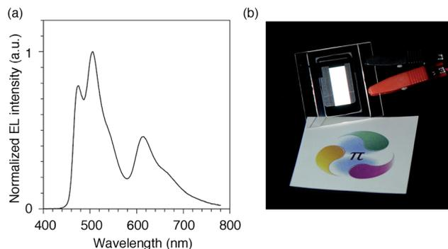
Fig. 9 White OLED with a single-layer architecture. (a) An electroluminescence spectrum at a current density of  $0.1 \text{ mA cm}^{-2}$ . (b) A picture of the device with an emitting area of  $16.6 \text{ mm} \times 6 \text{ mm}$ . The sheet under the device is showing a color reference printed on white paper, and the original colors can be found at <http://www.jst.go.jp/erato/isobe/>.
