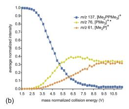
Fig. 2 Average normalized intensities of  $[R_2PPMe_3]^+$ ,  $[PMe_3]^+$  and  $[R_2P]^+$  (R = Ph (a) and Me (b)) as a function of mass normalized collision energy in ESI-CID-MS/MS experiments.
