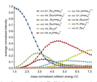
Fig. 1 Fragmentation plot for  $[^{t}Bu_{2}PPMe_{3}]^{+}$ . Average normalized intensities of  $[^{t}Bu_{2}PPMe_{3}]^{+}$  and its array of daughter fragments as a function of mass normalized collision energy in ESI-CID-MS/MS experiments.
