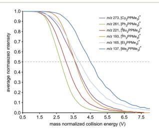
Fig. 4 The decay of  $[R_2PPMe_3]^+$  cations (R = Me, Et, <sup>i</sup>Pr, <sup>t</sup>Bu, Cy, Ph) in terms of average normalized intensities with increasing mass normalized collision energy. Dashed line indicates 50% disappearance.
