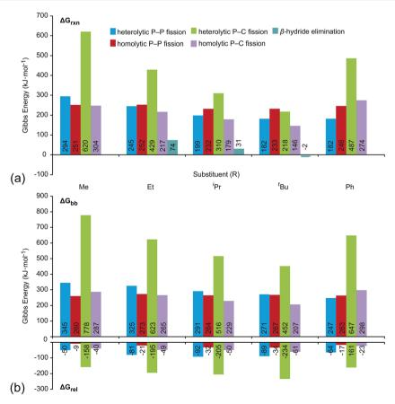
Fig. 6 (a) Gibbs energies of reaction ( $\Delta G_{rxn}$ ) for dissociation processes of  $[R_2PPMe_3]^+$  modelled in the gas-phase (298 K) at the PBE1PBE/6-311++G(d,p) level. See Scheme 2 for process definitions. (b) Decomposition of  $\Delta G_{rxn}$  into bond break ( $\Delta G_{bb}$ ) and fragment relaxation ( $\Delta G_{rel}$ ) Gibbs energies. All values given in kJ mol<sup>-1</sup>.
