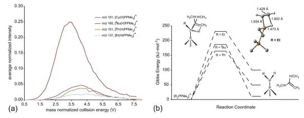
Fig. 7 (a) The average normalized intensities  $[R(H)PPMe_3]^+$  fragments formed through β-hydride elimination as a function of mass normalized collision energy. (b) Calculated (PBE1PBE/6-311++G(d,p)) reaction coordinate for β-hydride elimination from  $[R_2PPMe_3]^+$   $(R=Et, PPMe_3)^+$ .
