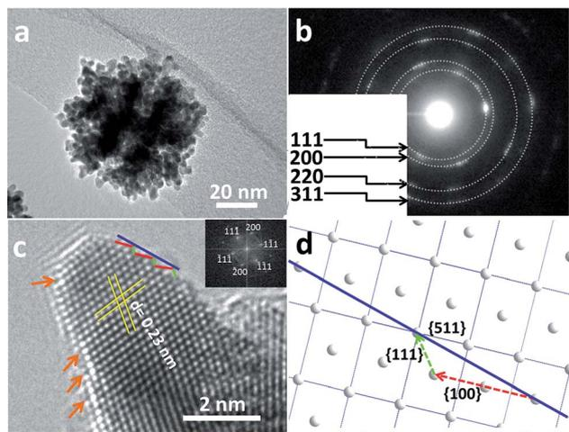
Fig. 3 (a) Typical TEM image and (b) the corresponding selected area ED pattern of a single MPN. (c) HRTEM image focused on the edge of Pt pore walls projected along the  $\langle 011 \rangle$  direction. (d) Schematic illustration for the exposed high-index facet. The inset image in panel (c) shows the corresponding FFT patterns of the HRTEM image.
