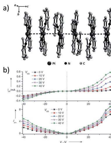
Fig. 9 (a) Crystal packing diagram of **61**·H<sub>2</sub>O. The PF<sub>6</sub><sup>−</sup> and water molecules are omitted for clarity. (b) Output characteristics ( $I_{\text{DS}}$  vs.  $V_{\text{DS}}$ ) and electroluminescence intensity ( $I$ ) of an OLEFET device with nanowires of **61** after annealing at 350 K (adapted with permission from ref. 112. Copyright 2008, Wiley-VCH Verlag GmbH & Co. KGaA).
