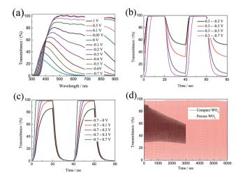
Fig. 4 (a) Transmittance of porous WO<sub>3</sub> film as a function of applied potential. (b and c) In situ optical responses of porous WO<sub>3</sub> films measured at 633 nm as a function of applied potential. (d) Cycle performance of the WO<sub>3</sub> films measured in 0.5 M H<sub>2</sub>SO<sub>4</sub> for 6000 s.
