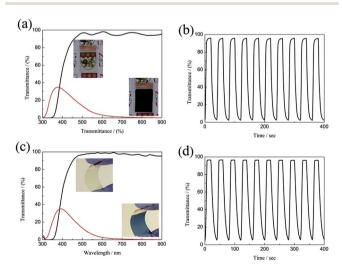
Fig. 5 Transmittance spectra and in situ optical responses of the WO<sub>3</sub> films on different substrates between the colored and bleached states: (a and b) FTO substrate. (c and d) ITO-PET substrate.
