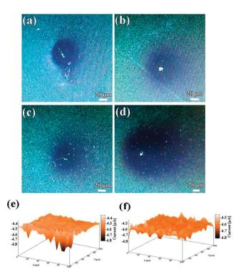
Fig. 6 Optical micrographs of the WO<sub>3</sub> in the surrounding of  $[Ru(NH_3)_6]^{2+}/[Ru(NH_3)_6]^{3+}$  redox mediator for 2 and 15 min: (a and b) compact WO<sub>3</sub> film, (c and d) porous WO<sub>3</sub> film. Electrochemical mappings of (e) compact WO<sub>3</sub> film, (f) porous WO<sub>3</sub> film.
