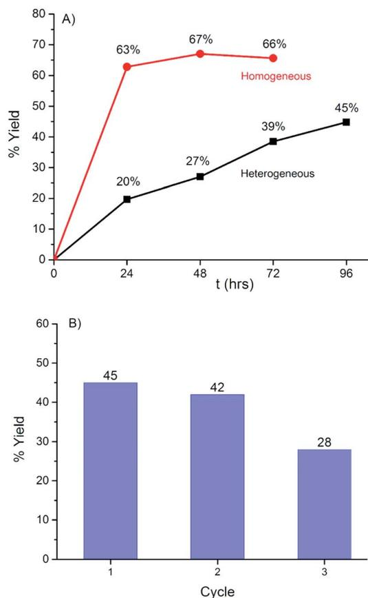
Fig. 8 (A) Yield vs. time plot of heterogeneous (black) and homogeneous (red) DA reaction under identical conditions (10 mol%  $[\text{Fe}]/[\text{MVK}]$  in  $\text{CH}_2\text{Cl}_2$ ,  $[\text{Iso}] = 0.4 \text{ M}$ ,  $[\text{MVK}] = 0.1 \text{ M}$ ). (B) Recycling of  $[(\text{Fp-L})_{0.6}(\text{TEA})_{2.4}][\text{In}_3(\text{BTC})_4]$  under the same conditions. Each cycle lasts 96 h.
