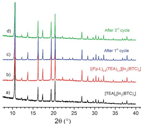
Fig. 6 Comparison of PXRD patterns between (a)  $[\text{TEA}]_3[\text{In}_3(\text{BTC})_4]$  and  $[(\text{Fp-L})_{0.6}(\text{TEA})_{2.4}][\text{In}_3(\text{BTC})_4]$  (b) as synthesized, (c) after one and (d) after three catalytic cycles.
