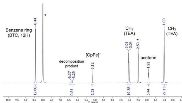
Fig. 7  $^1\text{H}$  NMR spectrum of  $[(\text{Fp-L})_{0.6}(\text{TEA})_{2.4}][\text{In}_3(\text{BTC})_4]$  after digestion in  $\text{DCl}/\text{d}^6\text{-dmsO}$  (1/5 v/v). NMR solvent peaks are marked with an asterisk.
