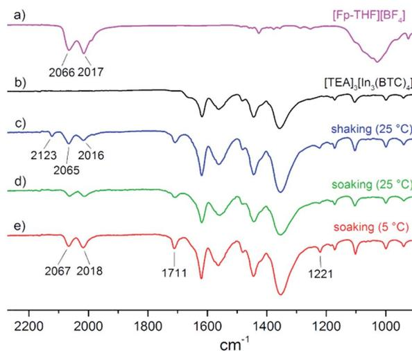
Fig. 5 Solid-state ATR IR spectra of (a)  $[\text{Fp-THF}][\text{BF}_4]$ , (b)  $[\text{TEA}]_3[\text{In}_3(\text{BTC})_4]$  and  $[(\text{Fp-L})_x(\text{TEA})_{3-x}][\text{In}_3(\text{BTC})_4]$  prepared *via* cation exchange in acetone under different conditions: (c) shaking for 1 day at 25 °C, (d) soaking for 1 day at 25 °C and (e) soaking for 2 days at 5 °C.
