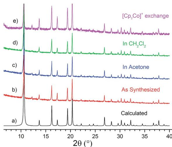
Fig. 1 Comparison of Powder X-ray Diffraction (PXRD) patterns of  $[\text{TEA}]_3[\text{In}_3(\text{BTC})_4]$ : (a) calculated from the single crystal structure, (b) as synthesized, (c) after soaking for one day at 298 K in acetone or (d)  $\text{CH}_2\text{Cl}_2$  and (e) after  $[\text{Cp}_2\text{Co}]^+$  cation exchange in acetone.
