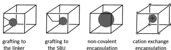
Scheme 1 Different methods for incorporating a TM catalyst (grey sphere) inside the pores of a MOF (cube).
