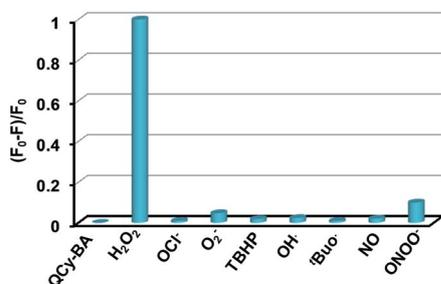
Fig. 2 Fluorescence response of **QCy-BA** (5  $\mu\text{M}$ ) to various reactive oxygen species (ROS) at an individual concentration of 100  $\mu\text{M}$ , where  $F_0$  and  $F$  are the fluorescence intensities of **QCy-BA** in the absence and presence of ROS, respectively.
