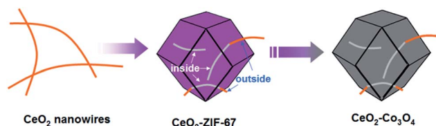
Fig. 1 The synthetic steps of short CeO 2 nanowires inserted porous Co 3 O 4 nanoframeworks.
