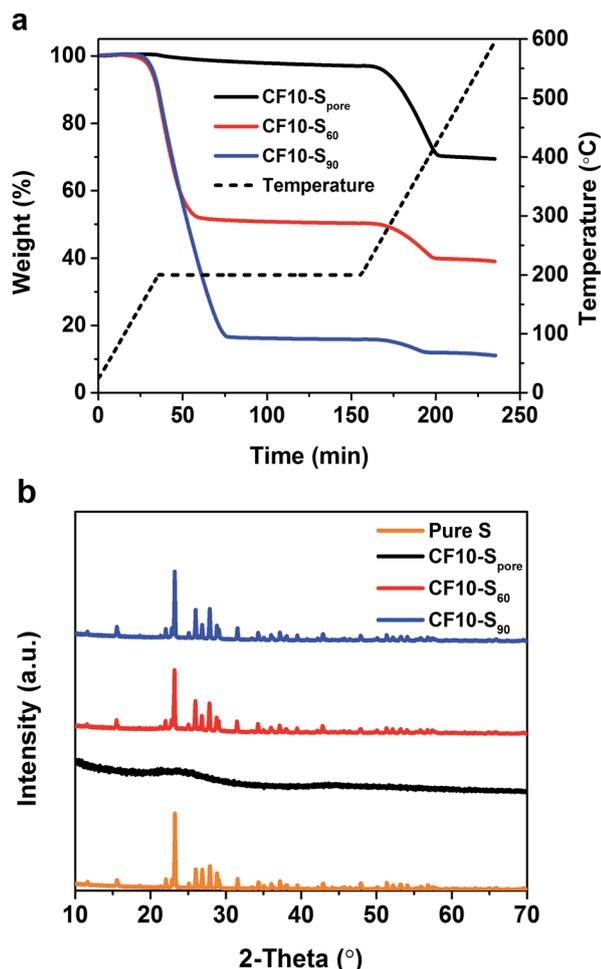
Fig. 2 (a) TGA curves and (b) XRD patterns of CF10-S<sub>pore</sub>, CF10-S<sub>60</sub> and CF10-S<sub>90</sub>.
