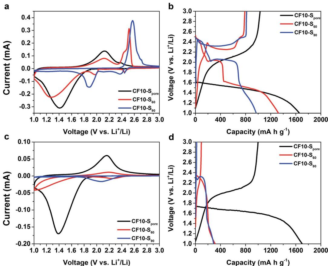
Fig. 3 The first CV scans at  $0.1 \text{ mV s}^{-1}$  and the first GCD curves at  $160 \text{ mA g}^{-1}$  of CF10-S<sub>pore</sub>, CF10-S<sub>60</sub>, and CF10-S<sub>90</sub> in TEGDME electrolyte (a) and (b) respectively, and in EC/DEC electrolyte (c) and (d), respectively.
