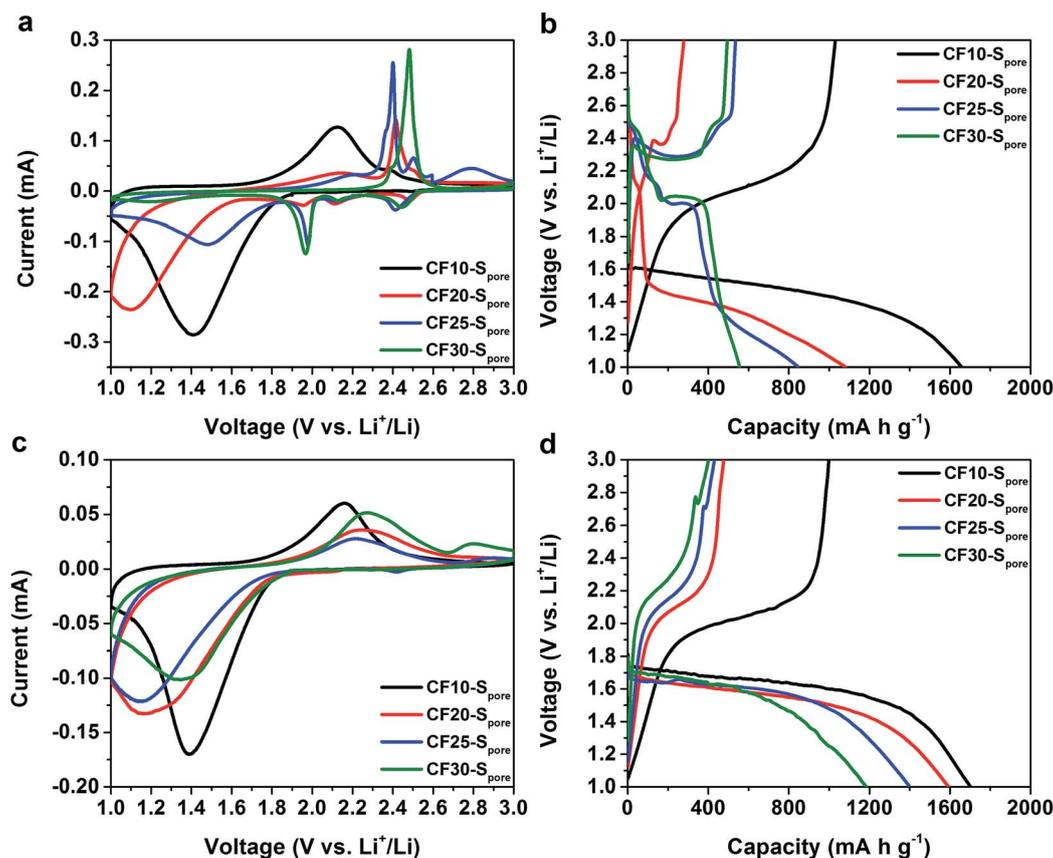
Fig. 5 The first CV scans at 0.1 mV s<sup>-1</sup> and GCD curves at 160 mA g<sup>-1</sup> of CF10-S<sub>pore</sub>, CF20-S<sub>pore</sub>, CF25-S<sub>pore</sub>, and CF30-S<sub>pore</sub> in TEGDME electrolyte (a) and (b) respectively, and in EC/DEC electrolyte (c) and (d), respectively.
