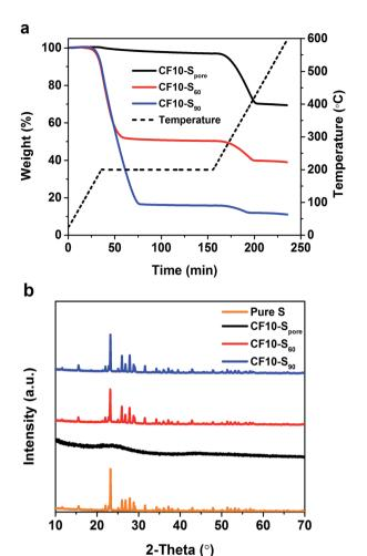
Fig. 2 (a) TGA curves and (b) XRD patterns of CF10–S  $_{\rm pore}$  , CF10–S  $_{\rm 60}$  and CF10–S  $_{\rm 90}$  .
