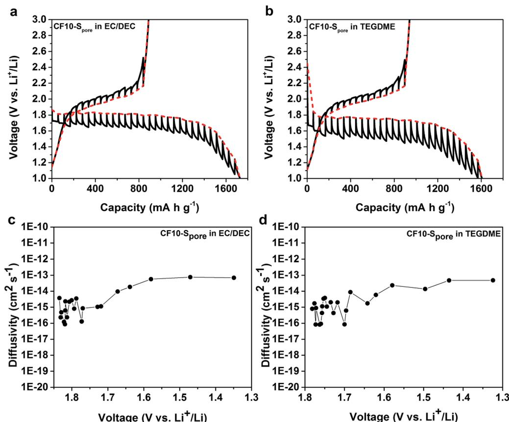
Fig. 6 GITT curves of CF10-S<sub>pore</sub> in (a) EC/DEC electrolyte and (b) TEGDME electrolyte; diffusivity of Li vs. potential calculated from the GITT data in (c) EC/DEC electrolyte and (d) TEGDME electrolyte.
