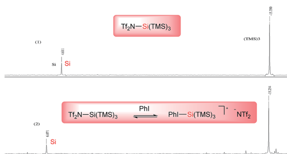
Scheme 2 ^{29}\text{Si} NMR study on the influence of iodobenzene on the aldol reaction. 1 equiv. of iodobenzene was used. Experiments conducted in NMR tube in \text{CD}_2\text{Cl}_2 under nitrogen atmosphere and at room temperature.
