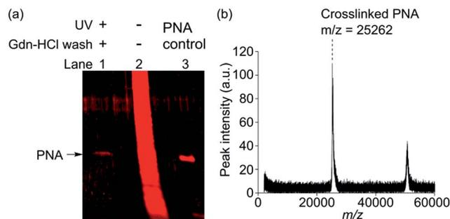
Fig. 3 Photoaffinity labeling of PNA (1  $\mu\text{g}$ , 50 nM) mixed in cell lysate (100  $\mu\text{g}$ , 0.5  $\text{mg mL}^{-1}$ ) using probe 2 (50 nM). (a) SDS-PAGE analysis showing protein band(s) eluted from probe 2. Lane 1: crosslinked-PNA enriched by Gdn-HCl wash, lane 2: negative control experiment with no UV irradiation and no Gdn-HCl wash, lane 3: PNA input as a control. (b) MALDI-TOF MS analysis showing the  $m/z$  peaks corresponding to PNA captured by probe 2.
