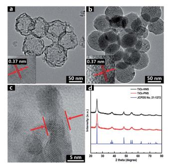
Fig. 2 TEM micrographs of (a)  $TiO_2$ -HNSs and (b)  $TiO_2$ -PNSs. (c) Spherical aberration corrected TEM micrograph of the  $TiO_2$ -HNS shell, and (d) XRD patterns of  $TiO_2$ -HNSs and  $TiO_2$ -PNSs.
