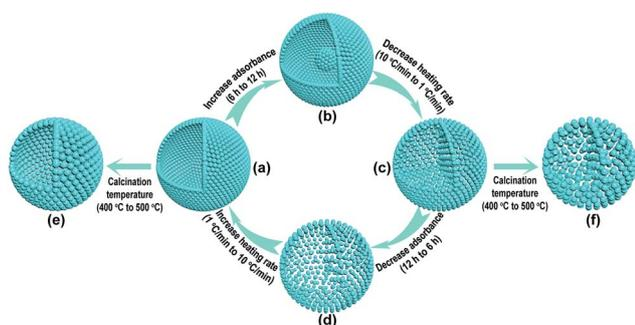
Fig. 1 Schematic diagram of the controllable synthesis for each product. (a)  $\text{TiO}_2$ -HNS; (b)  $\text{TiO}_2$ -core-shell; (c)  $\text{TiO}_2$ -PNS; (d)  $\text{TiO}_2$ -PNS-LS; (e)  $\text{TiO}_2$ -HNS-500 and (f)  $\text{TiO}_2$ -PNS-500.
