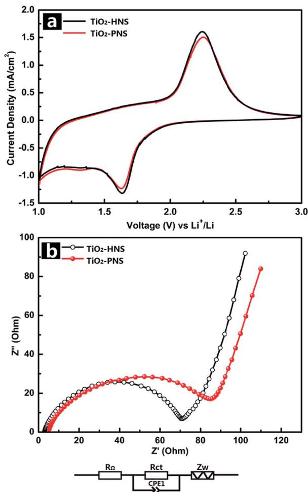
Fig. 4 (a) Cyclic voltammetry profiles of the TiO<sub>2</sub>-HNSs and TiO<sub>2</sub>-PNSs at a scan rate of 1 mV s<sup>-1</sup> between 1.0 V and 3.0 V for the first cycle, and (b) electrochemical impedance spectra (EIS) of the TiO<sub>2</sub>-HNSs and TiO<sub>2</sub>-PNSs ( $R_{\Omega}$ : external resistance,  $R_{ct}$ : charge transfer resistance, CPE1: constant phase element,  $Z_w$ : Warburg impedance).
