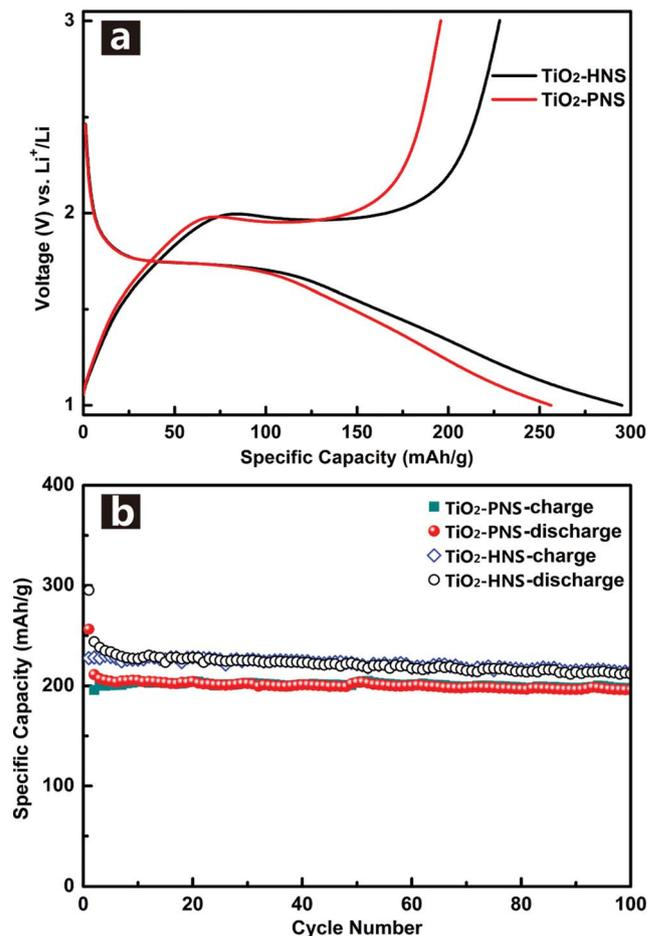
Fig. 5 (a) Initial charge–discharge voltage profiles and (b) cycling performance of the TiO<sub>2</sub>-HNSs and TiO<sub>2</sub>-PNS at a current rate of 1 C between 1.0 and 3.0 V.
