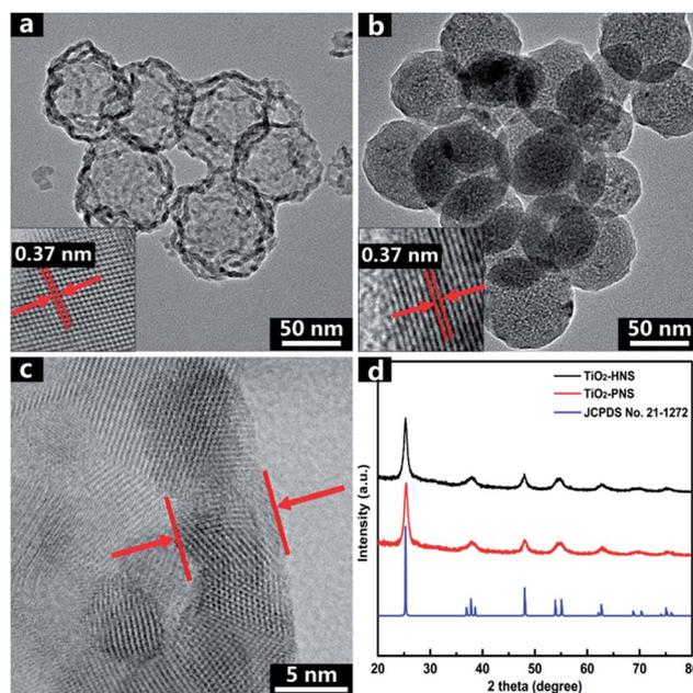
Fig. 2 TEM micrographs of (a)  $\text{TiO}_2$ -HNSs and (b)  $\text{TiO}_2$ -PNSs. (c) Spherical aberration corrected TEM micrograph of the  $\text{TiO}_2$ -HNS shell, and (d) XRD patterns of  $\text{TiO}_2$ -HNSs and  $\text{TiO}_2$ -PNSs.
