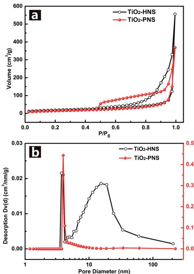
Fig. 3 (a) Nitrogen adsorption/desorption isotherms and (b) Barrett-Joyner-Halenda (BJH) pore-size distribution curves of the TiO<sub>2</sub>-HNS and TiO<sub>2</sub>-PNSs.
