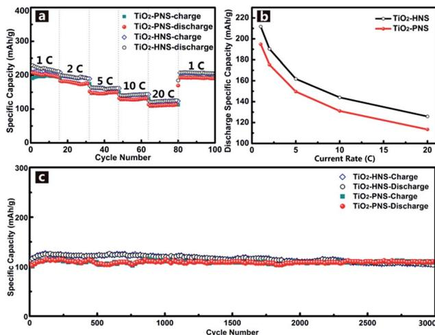
Fig. 6 (a) Cycling performance at various charge–discharge current rates of the TiO<sub>2</sub>-HNSs and TiO<sub>2</sub>-PNSs between 1.0 and 3.0 V. (b) Statistics of the discharge specific capacities at various current rates according to the rate performance in (a). (Each discharge capacity summarized here is the last cycle of each current rate.) (c) Long-term cycling performance of the TiO<sub>2</sub>-HNSs and TiO<sub>2</sub>-PNSs at a high current rate of 20 C for 3000 cycles.
