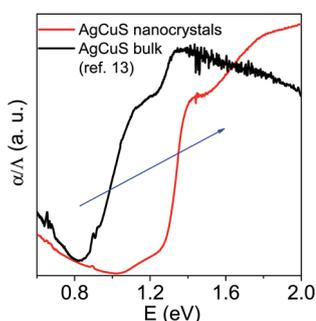
Fig. 8 Room temperature optical absorption spectra of as synthesized AgCuS nanocrystals (obtained after 30 min of reaction) compared with the previously reported bulk AgCuS.<sup>13</sup>
