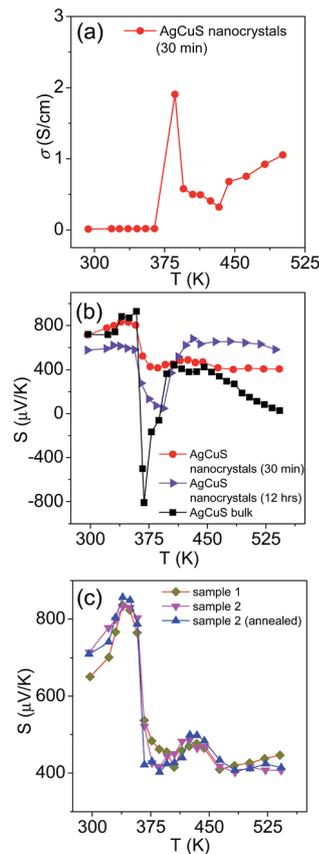
Fig. 7 (a) Temperature dependent electrical conductivity ( $\sigma$ ) of AgCuS nanocrystals obtained after 30 min of reaction. (b) Temperature dependent Seebeck coefficients ( $S$ ) of AgCuS nanocrystals obtained after 30 min and 12 h of reaction, which are compared to that of their bulk counterpart.<sup>13</sup> (c) Temperature dependent Seebeck coefficients ( $S$ ) of different batches of nanocrystalline AgCuS samples (30 min of reaction) show the reproducibility and temperature stability.
