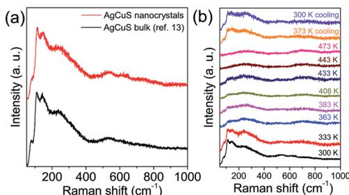
Fig. 6 (a) Room temperature Raman spectra of nanocrystalline AgCuS (obtained after 30 min of reaction) compared with that of the previously reported bulk AgCuS sample.<sup>13</sup> (b) Temperature dependent Raman spectra of nanocrystalline AgCuS (obtained after 30 min of reaction).
