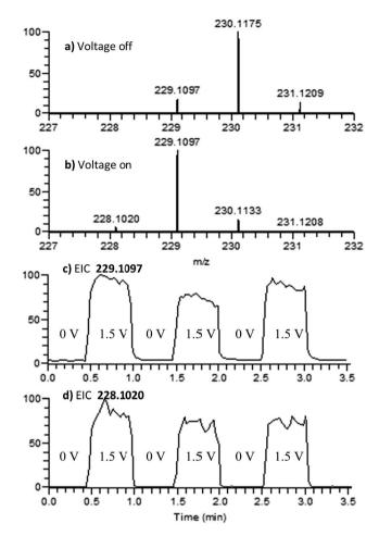
Fig. 3 Positive-ion mode mass spectra of DMDPA. (a) 0.0 V applied to the working electrode; (b) 1.5 V applied to the working electrode; (c) EIC for the 229.1097 peak as a function of the applied potential; and (d) EIC for the 228.1020 peak as a function of the applied potential.
