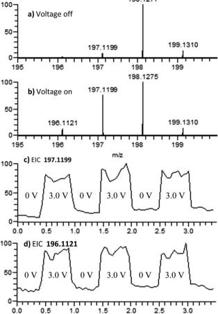
Fig. 4 Positive-ion mode mass spectra of DPTA. (a) 0.0 V applied to the working electrode; (b) 3.0 V applied to the working electrode; (c) EIC for the 197.1199 peak as a function of the applied potential; and (d) EIC for the 196.1121 peak as a function of the applied potential.
