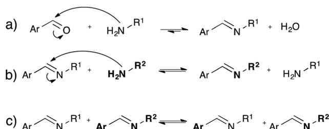
Fig. 10 Reversible processes associated with imine chemistry. (a) Equilibrium of imine formation, *via* intermediate hemi-aminal formation; (b) transamination between imines and amines *via* intermediate aminal formation; (c) imine metathesis.
