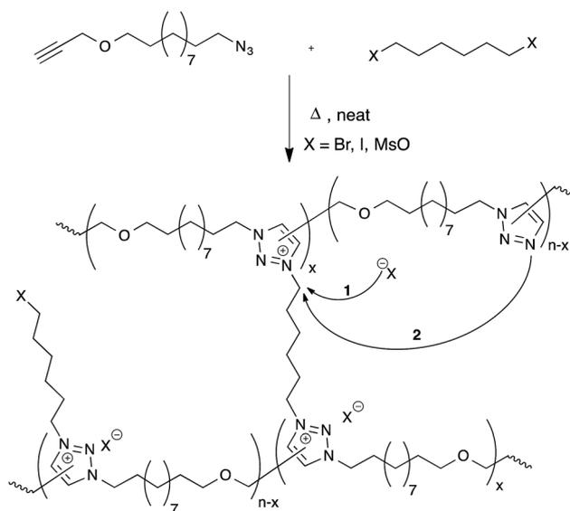
Fig. 6 Polymerisation of  $\alpha$ -azide- $\omega$ -alkyne monomers with bisfunctional alkylating agents results in polymer networks *via* the formation of 1,2,3-triazoles followed by the cross-linking process through alkylation to 1,2,3-triazoliums. The resulting networks can rearrange their topology through exchange between 1,2,3-triazoles and 1,2,3-triazoliums.
