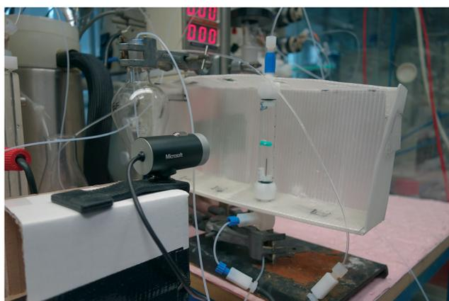
Fig. 6 An open-source machine vision system<sup>22–25</sup> was used to control the continuous extraction in Phase 2. The low-cost consumer web-camera detected the position of the green coloured float, sending information to a Raspberry Pi device which in turn sent commands to an Arduino board connected to a small peristaltic pump.
