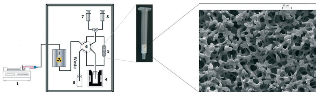
Fig. 1 Schematic representation of the monolith based system for <sup>68</sup>Ga processing and radiolabelling (left), photograph of cation-exchange silica-monolith column (centre) and SEM image of SiO<sub>2</sub> monolith-SO<sub>3</sub>H (right, scale bar: 20 μm).
