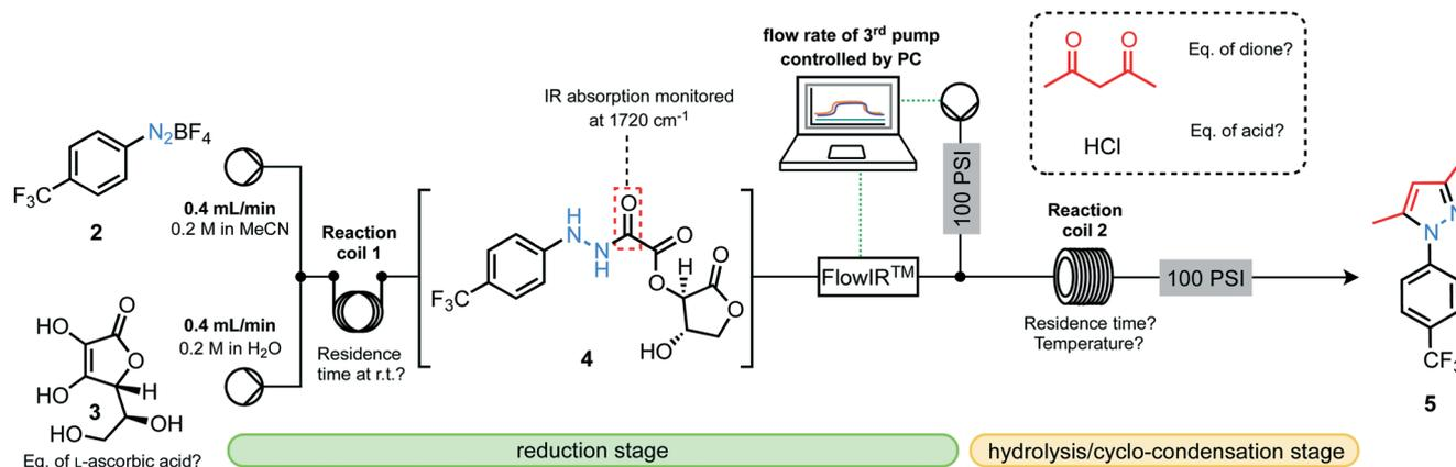
Fig. 2 Equipment setup for segmented flow reduction/hydrolysis/cyclo-condensation sequence.
