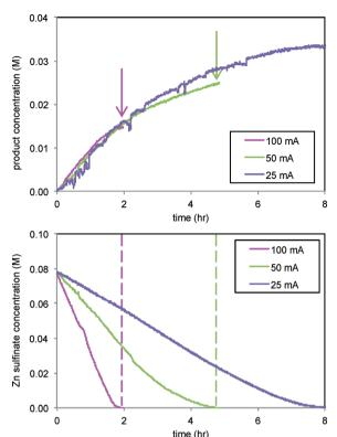
Fig. 7 Reaction of Scheme 2 carried out at different electrode currents. Top: Product 4 formation (1145 cm<sup>-1</sup>). Bottom: Consumption of Zn sulfinate (1722 cm<sup>-1</sup>). 3 equivalents of Zn sulfinate were employed compared to substrate 3.
