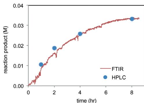
Fig. 4 Comparison of FTIR product **4** profile (peak at  $1145\text{ m}^{-1}$ ) with product **4** analysis by HPLC of sample aliquots in the reaction of Scheme 2.
