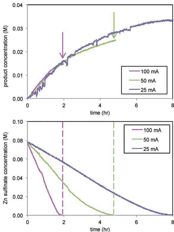
Fig. 7 Reaction of Scheme 2 carried out at different electrode currents. Top: Product 4 formation ( $1145 \text{ cm}^{-1}$ ). Bottom: Consumption of Zn sulfinate ( $1722 \text{ cm}^{-1}$ ). 3 equivalents of Zn sulfinate were employed compared to substrate 3.
