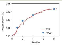
Fig. 4 Comparison of FTIR product 4 profile (peak at 1145 m<sup>-1</sup>) with product 4 analysis by HPLC of sample aliquots in the reaction of Scheme 2.
