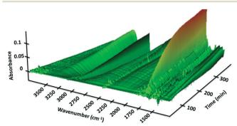
Fig. 3 FTIR spectra of the reaction of Scheme 1 as a function of wavenumber and reaction time carried out in the recycle reactor flowing through the FTIR transmission cell. Verbenone product 2 at  $1680 \text{ cm}^{-1}$ .  $[1]_0 = 40 \text{ mM}$ ;  $[TBHP]_0 = 200 \text{ mM}$ .
