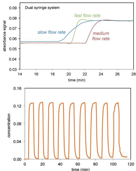
Fig. 2 FTIR monitoring of injections of the verbenone 2 signal ( $1680\text{ cm}^{-1}$ ) into solvent in recycle flow through the electrochemical cell and the FTIR flow cell system as shown in Scheme 3 and Fig. 1. Top: Three different flow rates for infusion/withdrawal in the syringe system (in  $\text{ml min}^{-1}$ ). Slow = 4/6; medium = 5/7; fast = 6/8. Bottom: Consecutive fast switching between streams of solvent and verbenone 2.
