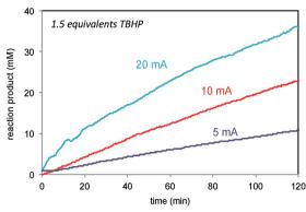
Fig. 6 Reaction of Scheme 1 carried out at different currents and TBHP concentrations. Top: 5 equivalents TBHP and 5, 10 20 mA current. Control experiments employing either no TBHP or no current are also shown. Bottom: 1.5 equivalents TBHP and 5, 10, and 20 mA current.
