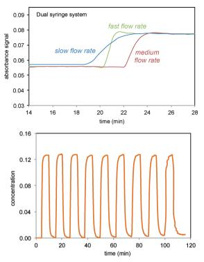
Fig. 2 FTIR monitoring of injections of the verbenone 2 signal (1680 cm<sup>-1</sup>) into solvent in recycle flow through the electrochemical cell and the FTIR flow cell system as shown in Scheme 3 and Fig. 1. Top: Three different flow rates for infusion/withdrawal in the syringe system (in ml  $min^{-1}$ ). Slow = 4/6; medium = 5/7; fast = 6/8. Bottom: Consecutive fast switching between streams of solvent and verbenone 2.
