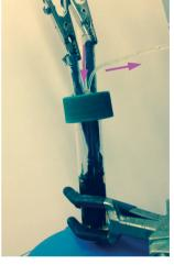
Fig. 1 Left: Flow-through FTIR cell for transmission FTIR spectroscopic monitoring of the electrochemical reactions of Schemes 1 and 2; Right: electrochemical cell with carbon cloth electrodes. Total solution volume = 8.2 ml; lines and syringes = 2.5 ml; syringe infusion/ withdrawal volume = 1 ml. Working solution volume in reactor during recycle flow = 5.7 ml.
