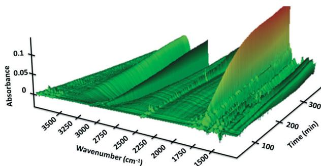
Fig. 3 FTIR spectra of the reaction of Scheme 1 as a function of wavenumber and reaction time carried out in the recycle reactor flowing through the FTIR transmission cell. Verbenone product 2 at  $1680\text{ cm}^{-1}$ .  $[1]_0 = 40\text{ mM}$ ;  $[\text{TBHP}]_0 = 200\text{ mM}$ .
