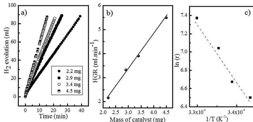
Fig. 5 Catalytic tests for the  $\text{Co}_{50}\text{C}_{100}$  sample: (a) hydrogen evolution curves for the catalyzed SBH hydrolysis. (b) Hydrogen generation rate as a function of the mass of the catalyst. (c) Arrhenius plot.
