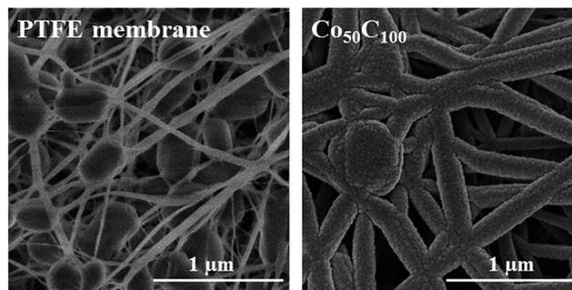
Fig. 8 SEM images of the PTFE membrane before (left) and after (right) deposition of the Co<sub>50</sub>C<sub>100</sub> coating.
