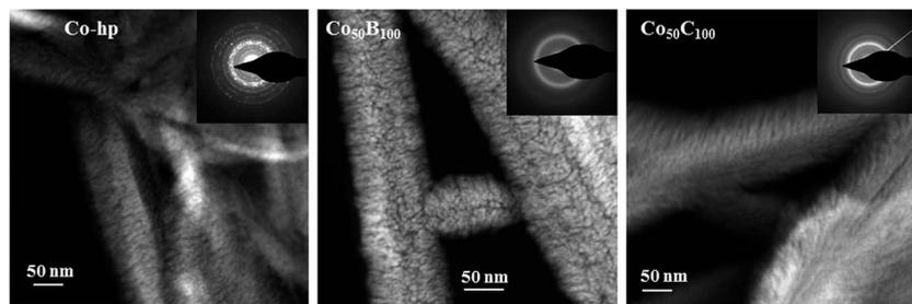
Fig. 9 STEM-HAADF images for selected coatings ( $\text{Co}_{50}\text{-hp}$ ,  $\text{Co}_{50}\text{B}_{100}$  and  $\text{Co}_{50}\text{C}_{100}$ ) deposited on the PTFE membrane fibers. The corresponding electron diffraction patterns are included as insets.
