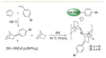
**Scheme 1** Synthesis and polymerization of  $\mathbf{1}$  to give p-bromophenyl-VA-PNBs.
