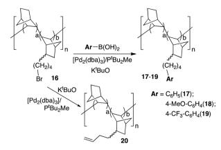
Scheme 4 Functionalization of VA-PNB 16 by Suzuki coupling and Pd-catalyzed  $\beta$ -H elimination.
