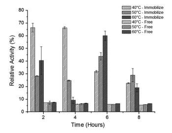
Fig. 2 Thermal stability at 40, 50 and 60 °C of free and immobilized CalB lipase in PEGylated poly(urea-urethane) nanoparticles.<sup>55</sup> This figure has been reproduced from ref: E. P. Cipolatti, A. Valério, G. Nicoletti, E. Theilacker, P. H. H. Araújo, C. Sayer, J. L. Ninow and D. de Oliveira, *J. Mol. Catal. B Enzym.*, 2014, **109**, 116–121 with permission from Pan Stanford Publishing.
