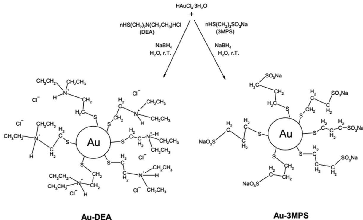
Fig. 7 Schematic synthesis of AuNPs stabilized with DEA and 3MPS.<sup>96</sup> This figure has been reproduced from ref: I. Venditti, C. Palocci, L. Chronopoulou, I. Fratoddi, L. Fontana, M. Diociaiuti and M. Vittoria, 2015, **131**, 93–101 with permission from Elsevier.
