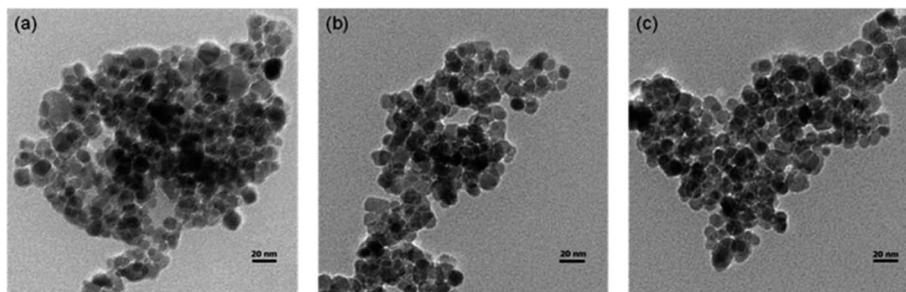
Fig. 3 TEM images of Fe<sub>3</sub>O<sub>4</sub> (a), Fe<sub>3</sub>O<sub>4</sub>-chitosan (b) and immobilized cellulase (c).<sup>61</sup> This figure has been reproduced from ref: L. Zang, J. Qiu, X. Wu, W. Zhang, E. Sakai and Y. Wei, *Ind. Eng. Chem. Res.*, 2014, **53**, 3448–3454 with permission from American Chemical Society.
