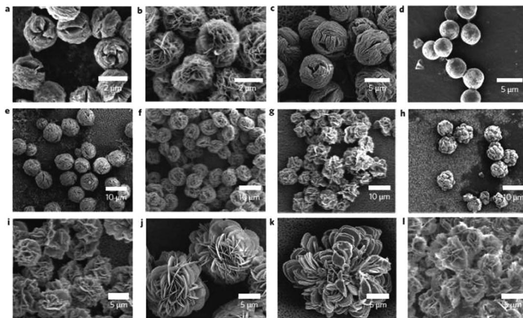
Fig. 8 SEM images of hybrid nanoflowers (a–l). Column 1,  $\alpha$ -lactalbumin; column 2, laccase; column 3, carbonic anhydrase; column 4, lipase; at protein concentrations of  $0.5 \text{ mg ml}^{-1}$  (a–d),  $0.1 \text{ mg ml}^{-1}$  (e–h) and  $0.02 \text{ mg ml}^{-1}$  (i–l)<sup>108a</sup>. This figure has reproduced from ref: J. Ge, J. Lei and R. N. Zare, *Nat. Nanotechnol.*, 2012, 7, 428–43 with permission from Nature Publishing Group.
