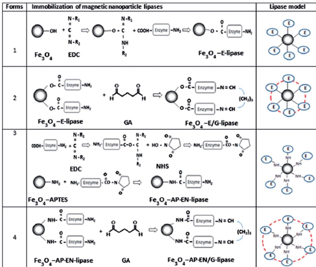
Fig. 6 Schematic diagram of magnetic nanoparticle lipase immobilization methods.<sup>44</sup> This figure has been reproduced from ref: M. Raita, J. Arnthong, V. Champreda and N. Laosiripojana, *Fuel Process. Technol.*, 2015, 134, 189–197 with permission from Elsevier.
