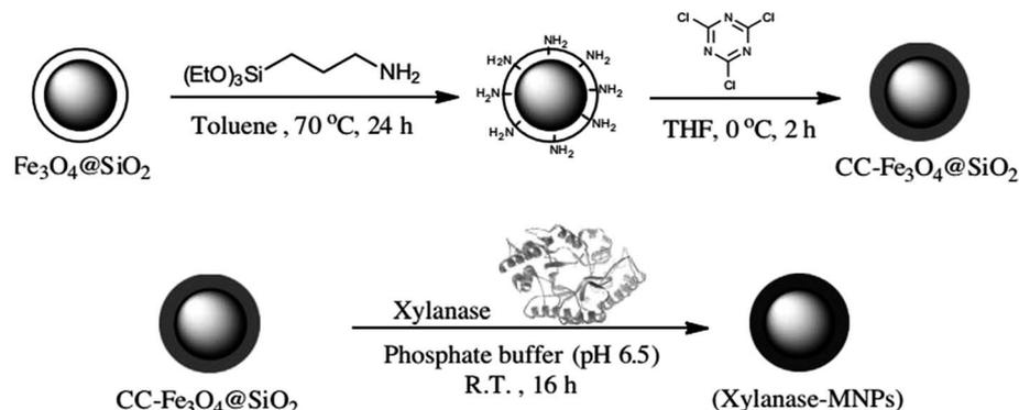
Fig. 5 Schematic representation of the method for covalently immobilization of xylanase on functionalized magnetic nanoparticles.<sup>72</sup> This figure has been reproduced from ref: A. Soozanipour, A. Taheri-Kafrani and A. Landarani Isfahani, *Chem. Eng. J.*, 2015, 270, 235–243 with permission from Elsevier.
