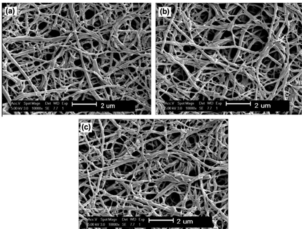
Fig. 4 SEM images of (a) original PVA-co-PE nanofibrous membrane, (b) lipase immobilized on PVA-co-PE nanofibrous membrane and (c) lipase immobilized on PVA-co-PE nanofibrous membrane after catalytic reactions.<sup>51</sup> This figure has been reproduced from ref: J. Zhu and G. Sun, *React. Funct. Polym.*, 2012, 72, 839–845 with permission from Elsevier.
